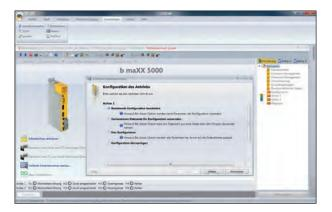
With the b maXX softdrivePLC Baumüller combines motion control and SPS functions in the controller and makes separate control hardware unnecessary for some applications.
