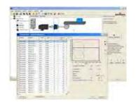
All standard functionalities of the Baumüller drives are stored in a data record in sizemaXX. They are always up-to-date and available to the user since the database can always be updated online. This allows for easily, quickly and precisely configuring complete drive groups. Up to six drive units, consisting of motor and converter, can be dimensioned in an interconnected system.
